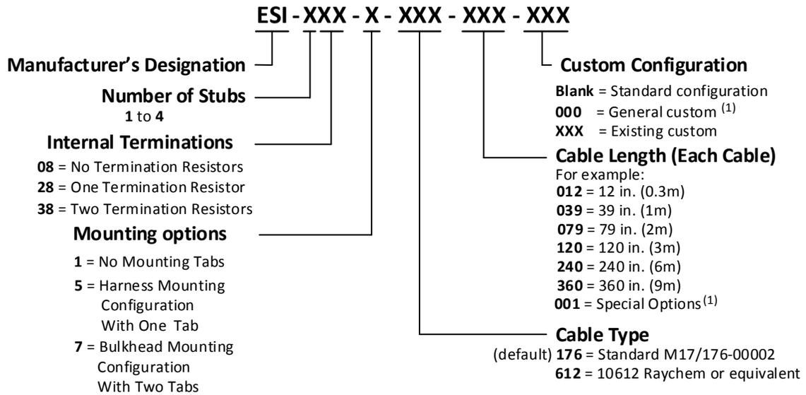
**Example:** ESI-408-1-176-039 is the part number for a four stub coupler with no internal termination resistor, no mounting tab, M17/176 cable, 1 meter length.
